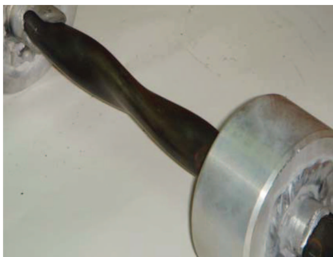
Figure 4 Photograph of the twisted tube with aluminum inlet block. (Color figure available online.)
